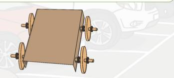
In this picture, the chassis is an upside down shoebox lid. Holes have been made on each side of the box and the axles have been threaded through.
